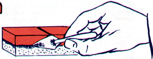
FIG. 3 After excess mortar dries, take trowel and trim it off as indicated above.
